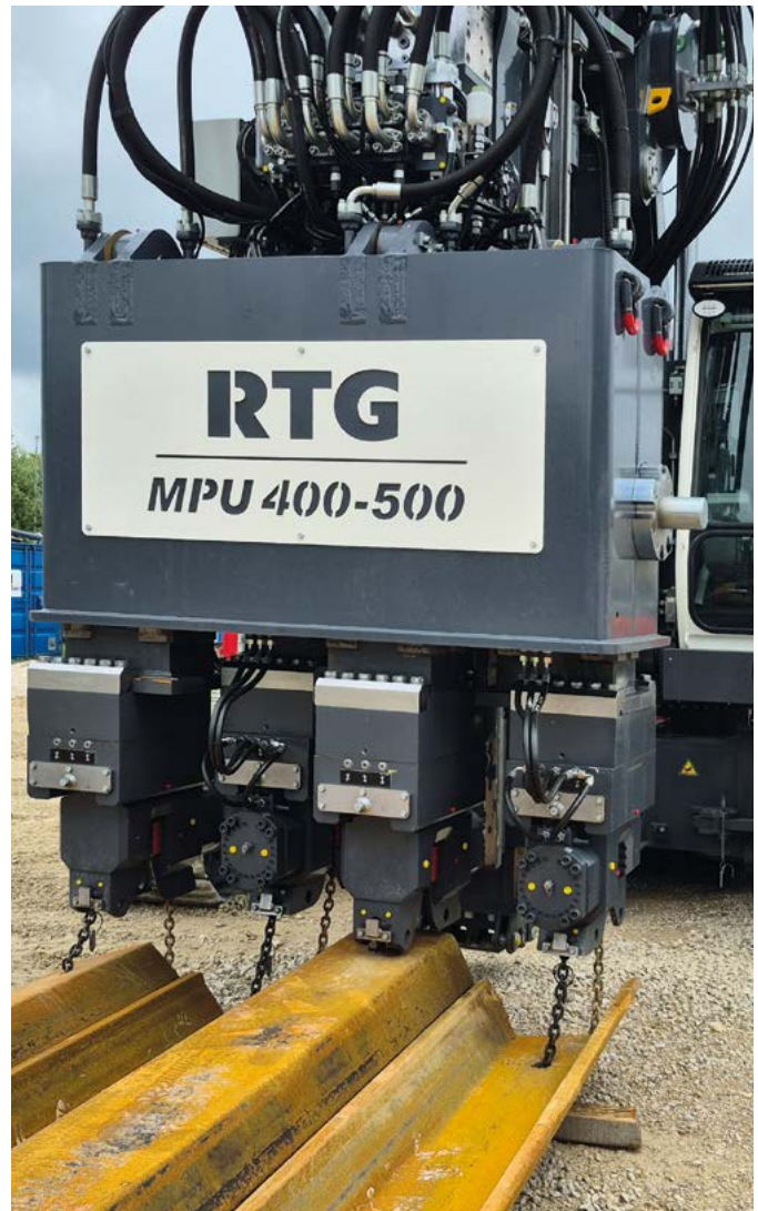
Spundwand-Pressen Sheet Pile Pressing
